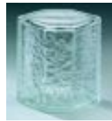
HEDRON® Corner Block, DECORA® and IceScapes® Patterns Hexagonal corner unit allows you to form 90° corners resulting in a gently rounded continuous glass face. The block can be used in combination with any other finishing unit.
